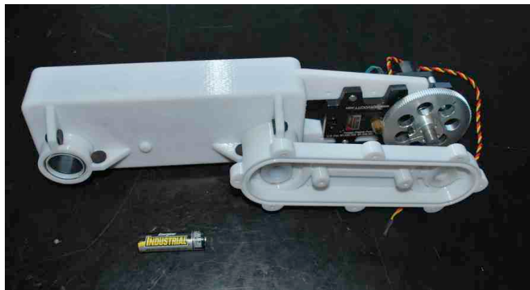
Figure 3.3: Picture of MONTe's drive assembly attached to half of a radial arm
