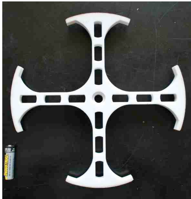
Figure 3.4: Picture of MONTe's initial Whег™ design
