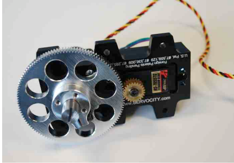
Figure 3.8: A picture of the high torque servo drive mechanism
