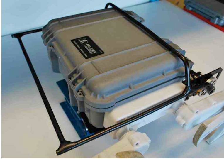
Figure 3.6: A picture of MONTe with the tail in the stowed position
