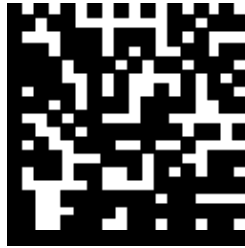
Figure 12. There Exists a Wide Range of Different 2D Matrix Code Types; This Figure Shows a Data Matrix ECC 200 Code. 54
