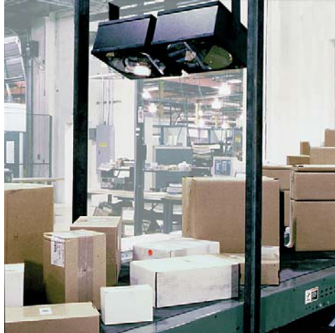
Figure 14. Fixed Barcode Scanner in a Conveyer Belt Application. 63
