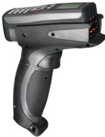
Figure 15. Handheld 2D Matrix Reader with USB and Bluetooth Connections. 66
