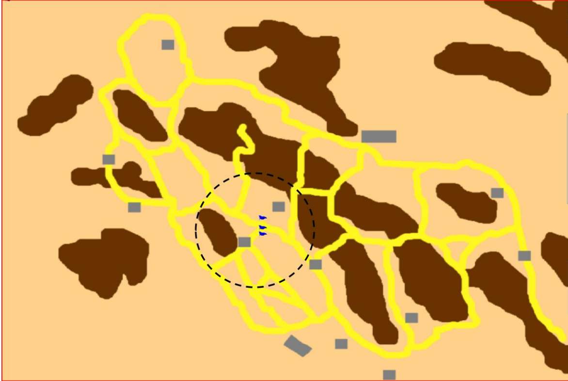
Figure 3. This is the MANA rendering of the same area as shown in Figure 2. The dark brown areas are elevations, the grey rectangles are urban terrain, and the yellow bands are the road network. Since MANA does not handle irregular boundaries well, a circle has been utilized to represent the Quackenbush Range. The blue flags are a MANA artifact and should be ignored.
