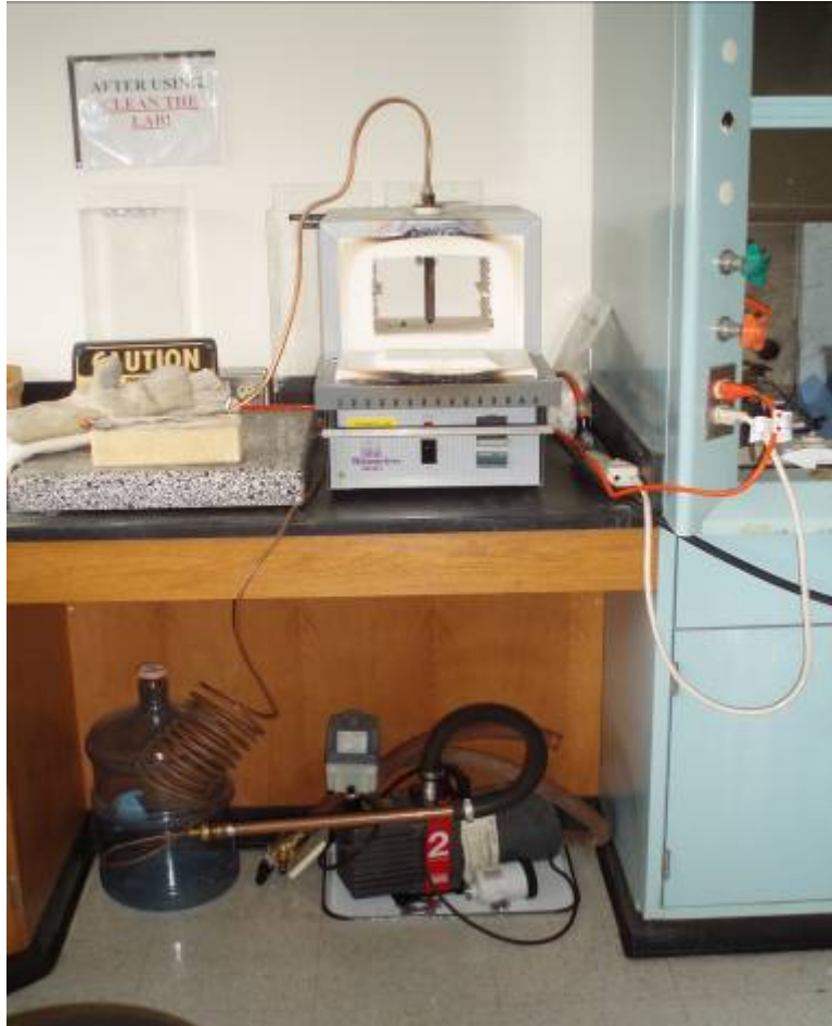
Figure 4. Photograph of the assembled argon purged furnace. The vacuum pump is seen below the counter.
