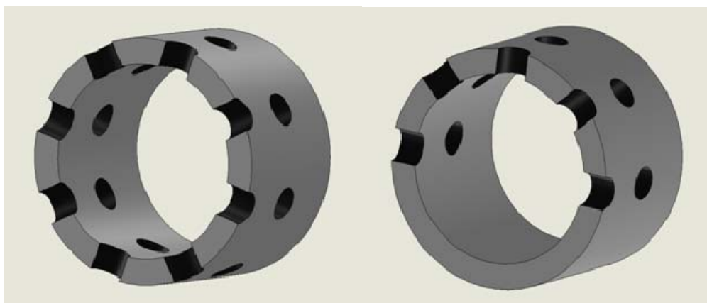
Figure 8. Comparison of Shroud Design With 360° Holes and 180° Holes
