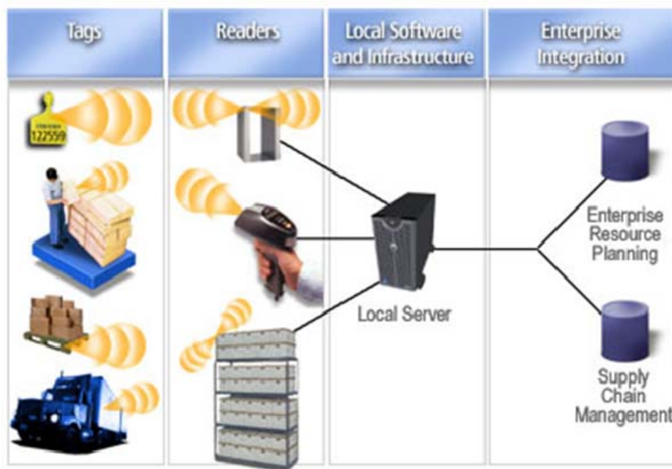
Figure 2. RFID system (From: Digitivity, 2008)
