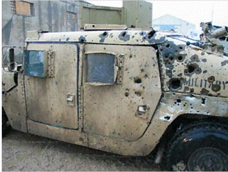
Figure 3. HUMVEE damaged by an EFP
