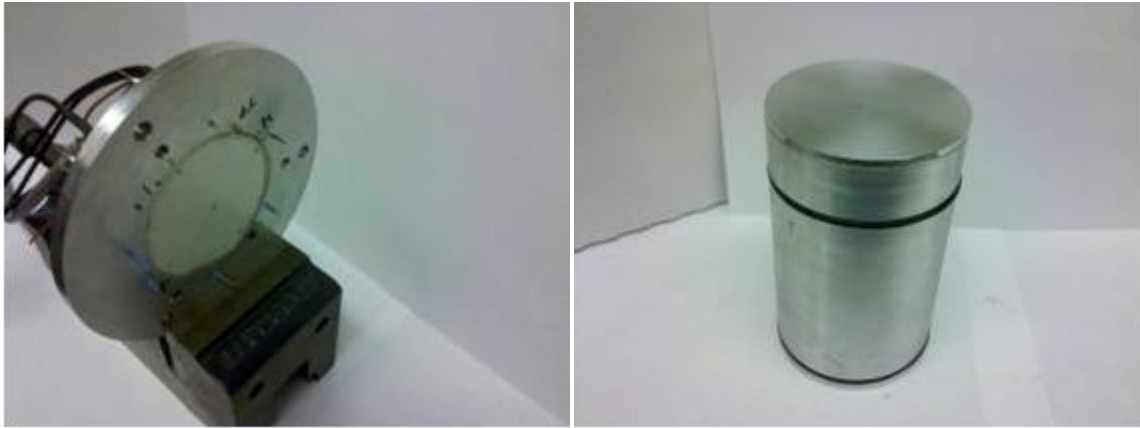
Figure 49. NPS Shot #10_15 target and projectile final assembly
