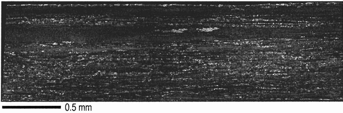
Figure 14. Rolling-direction inverse-pole-figure map of sample 5C9-1XR with image-quality overlay.
