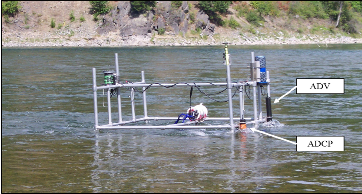
Figure 3. Picture of frame with ECM array (not visible), ADV, and ADCP deployed in the Kootenai River, ID.
