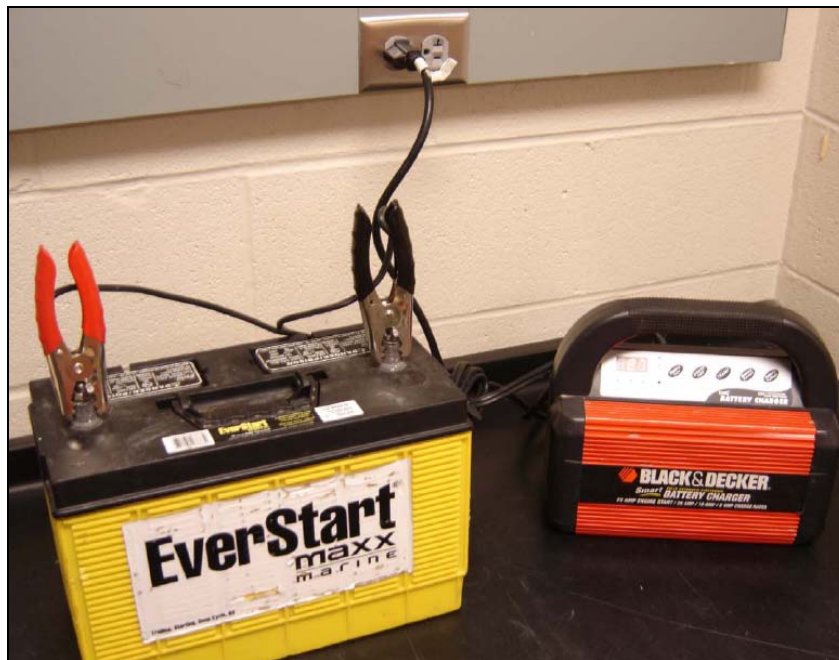
Figure A.1: 2 each 12 volt marine batteries should be charged before each survey.
