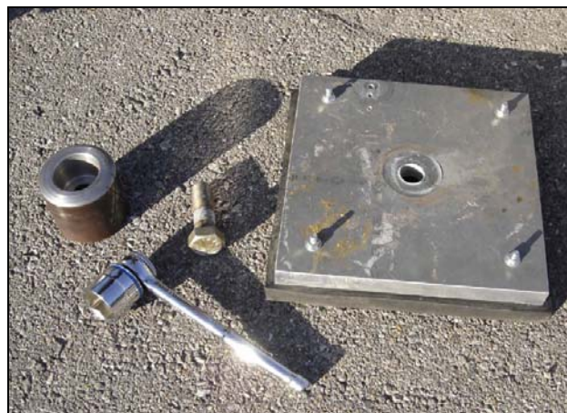
Figure A.8: Picture of the hammer (left) and rubber (right) foot. The Wrench with 1.5 inch socket is used to attach either foot to the impact arm using the attachment bolt.
