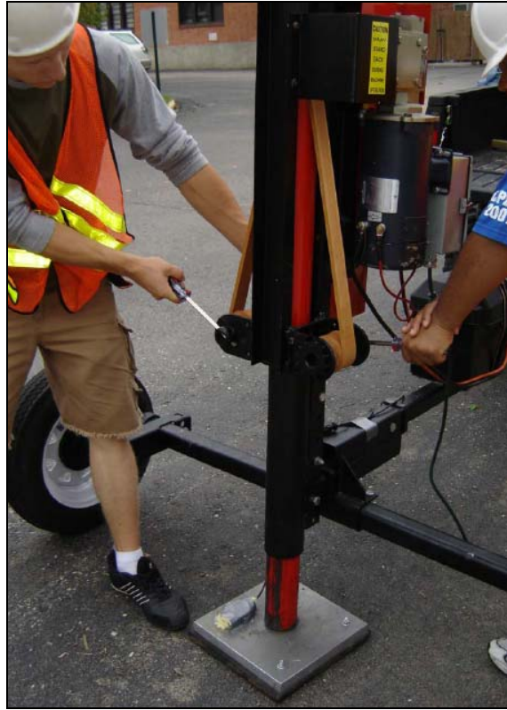
Figure A.9: The Elastomere band is threaded through the top of the arm and opposing cranks that are then tightened in parallel with 18” screwdrivers.
