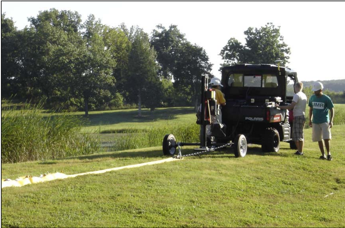
Figure 1: The mobile seismic unit in operation at Ber Juan Park test site.
