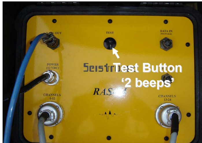
Figure A.18: Once all the systems are connected and turned on, pressing the button on the RAS-24 should return '2 beeps'. 2 beeps means the system is connected. 1 beep means there is a disconnected, misrouted, or damaged cable / cable connector.
