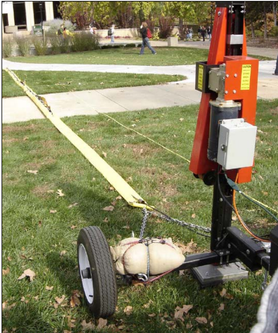
Figure 3.8: The seismic impact source that imparts seismic energy into the ground is an active seismic system. The energy propagates through the ground and is measured by the geophones embedded along the yellow firehouse streamer. Note the rubberized foot configuration as to avoid damaging the thin concrete sidewalk.
