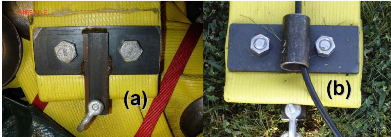
Figure B.7: (a) Bottom of streamer towing clamp with anchor shackle used to drag the streamer, (b) upper portion of streamer towing clamp with pipe to route geophone cable.
