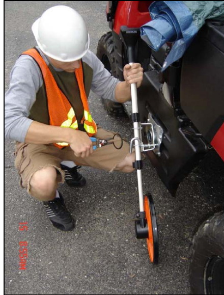
Figure A.13: Attaching the Digi-roller to the rotating adapter housing on the ATV.
