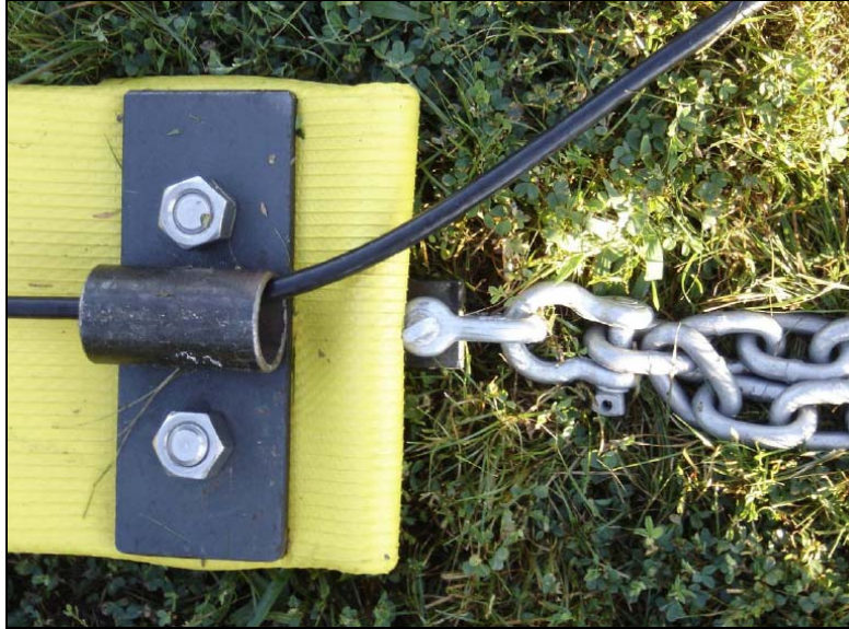
Figure A.6: 2 metal shackles that connect the streamer towing clamp to the array tow chain.
