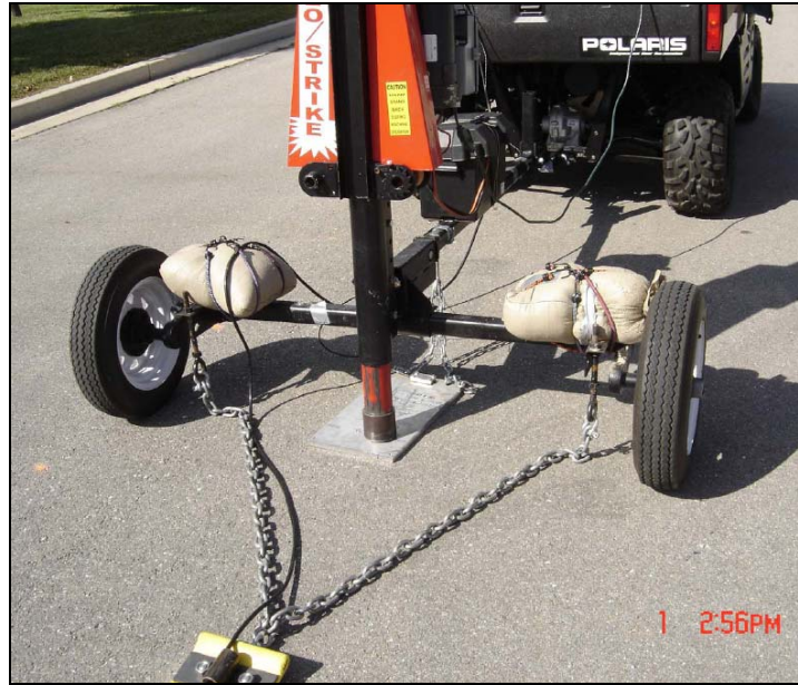
Figure A.10: Seismic Impact Source (GEO-Strike) Trailer configured with plate and hammer head. Sandbags weighted the chassis such that when the source was used, the trailer was not lifted off the ground.
