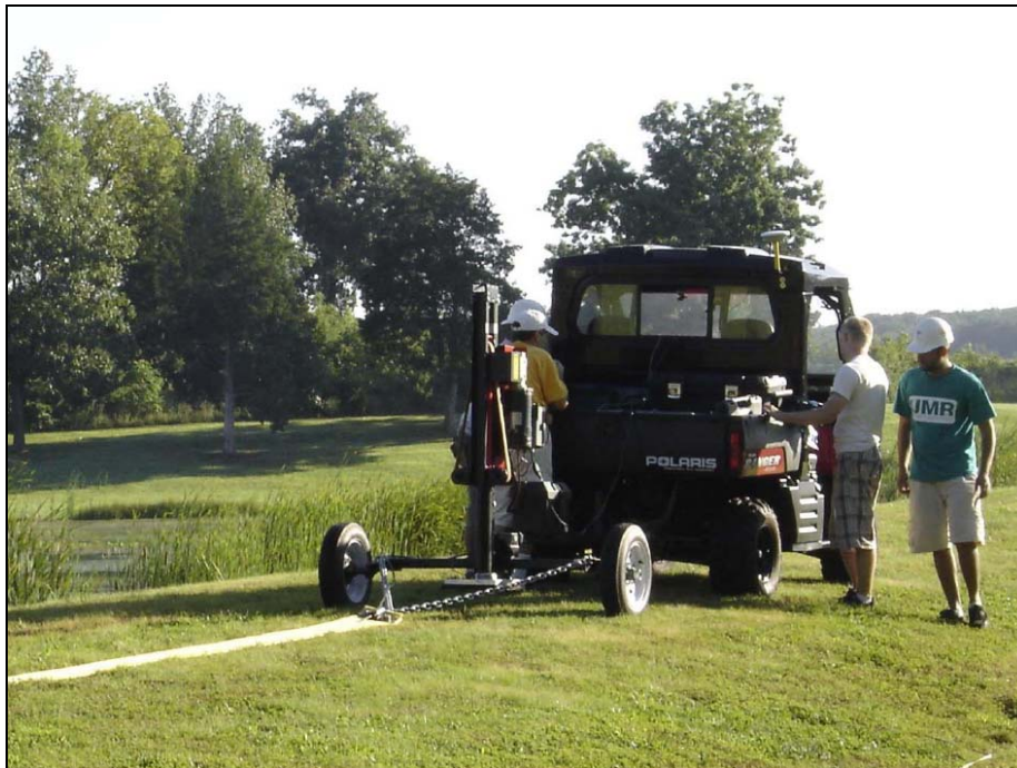
Figure 1.1: Demonstration Mobile Seismic Unit (DMSU) designed to rapidly and reliably locate shallow man-made subterranean passageways.
