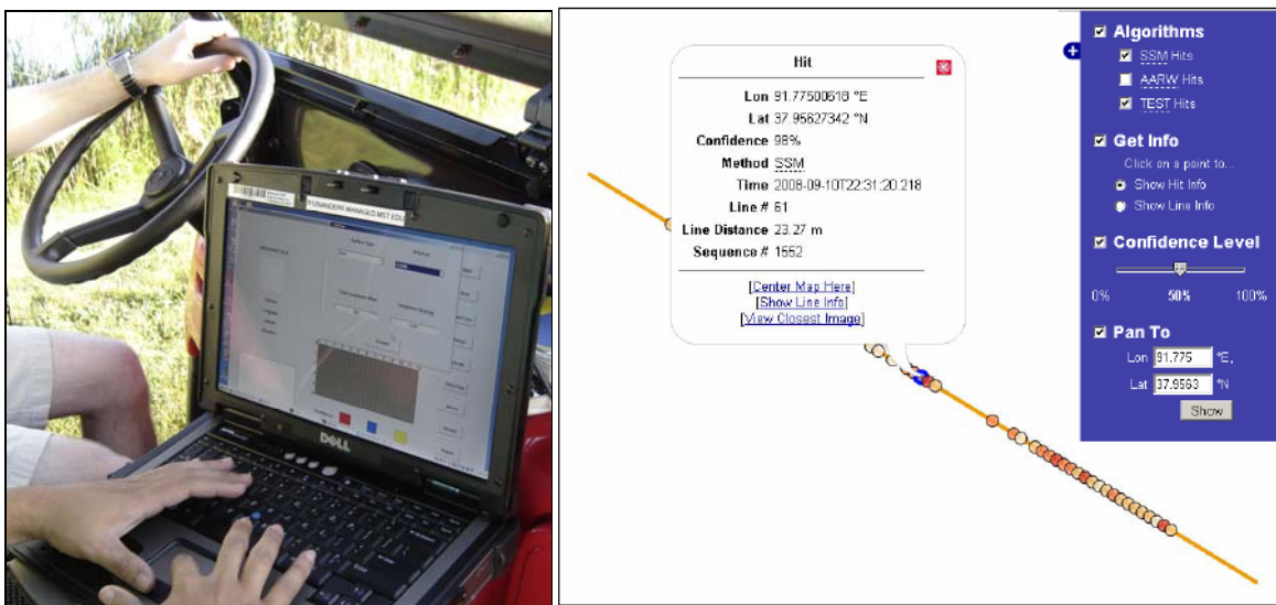
Figure 2: (a) Laptop with Seismic Interpretation Software. The operator is entering field parameters. (b) Mapping Tool (Screen Capture). Displays location of probable tunnel(s) based on automated interpretation of the field data.
