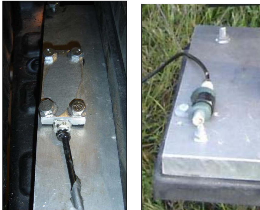
Figure B.6: The metal plate (for soft soil) has an aluminum bracket with a core semi-circular groove that clamps the trigger using standard bolts (left). The rubber foot uses a clamp with foam insulation to house the trigger (right).
