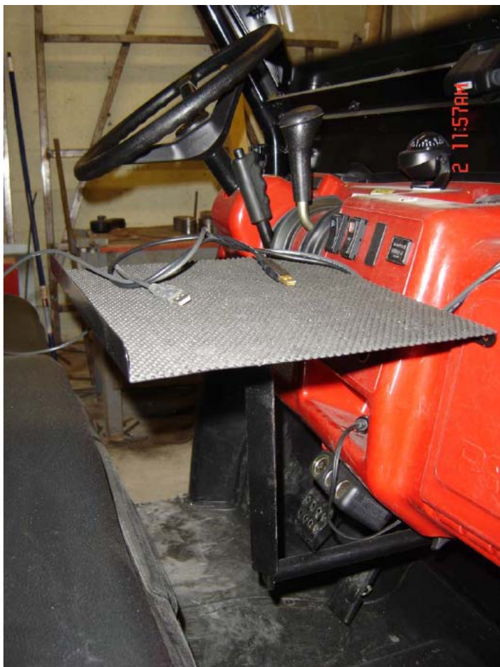
Figure B.4: Law Enforcement Laptop Kit. Note 3-way 12V outlet power adapter and extended USB cables that plug into the back of the Dell XFR D630 Toughbook.
