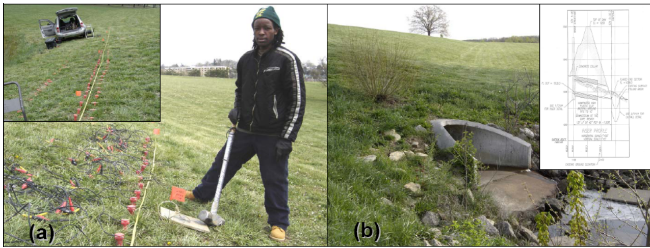
Figure 3.3: (a) 4.5 Hz geophone array over a tunnel structure at a Ber Juan Park in Rolla, Mo.: Graduate student Amos Wamweya assists by striking a sledge hammer to a plate on the ground that generates the seismic energy that will be measured by the geophones. (b) Cross-section blueprint and on site survey measurements of the Ber Juan spillway tunnel is compared to the geophysical field data to determine agreement of approximated void location using the respective Rayleigh Wave geophysical cross section(s).
