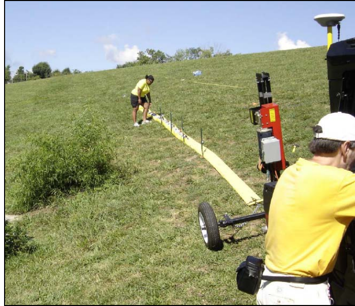
Figure A.3: Missouri S&T Student Janelly Griffith secures pickets to guide the streamer array on a slope. Terrain with slopes / slippery surfaces (hillside with wet grass) will cause the streamer array to slide down slope diagonally (parallel direction to maximum slope). Short pickets were used to hold the streamer on the survey line trajectory.
