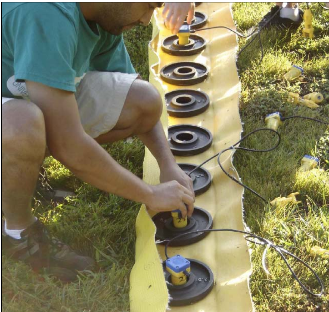
Figure 3.7: Missouri S&T Graduate Student Preetam Modur screws a geophone into the geophone plate. A firehose acts as a semi-rigid construct where a cast iron weight was spot welded to the top of the geophone adapter plate. As the project progressed, a second cast iron weight was added.
