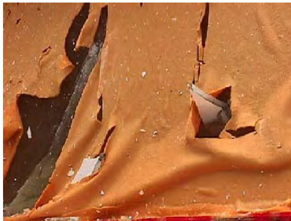
Figure 3. Annealed Shards Embedded in Ballistic Gelatin from a Multi-Hit Test
