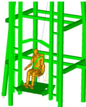
Nested seating system design for blastworthiness modeling and optimization
