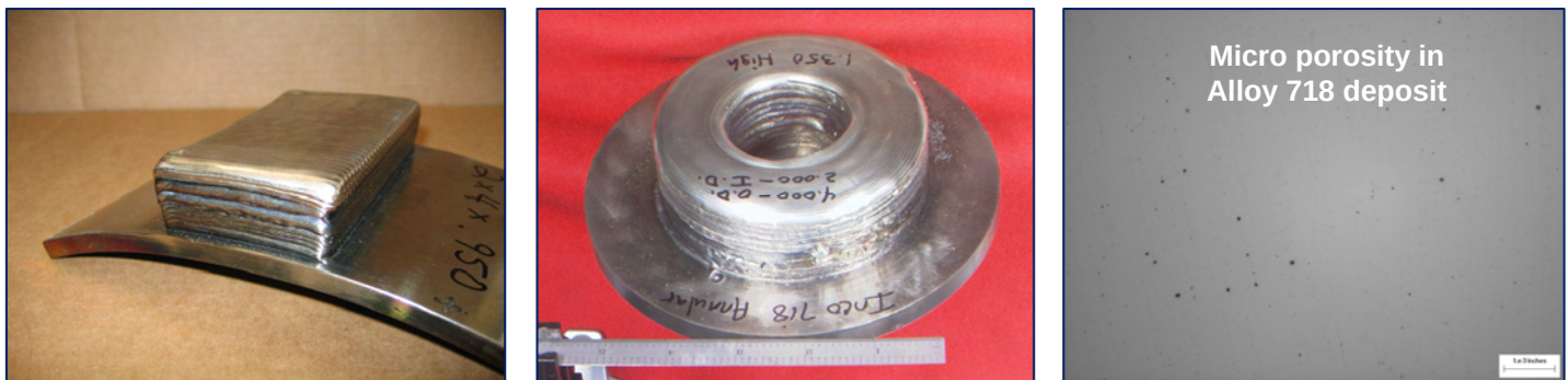
Figure 3: EBWD Deposits on Alloy 718
