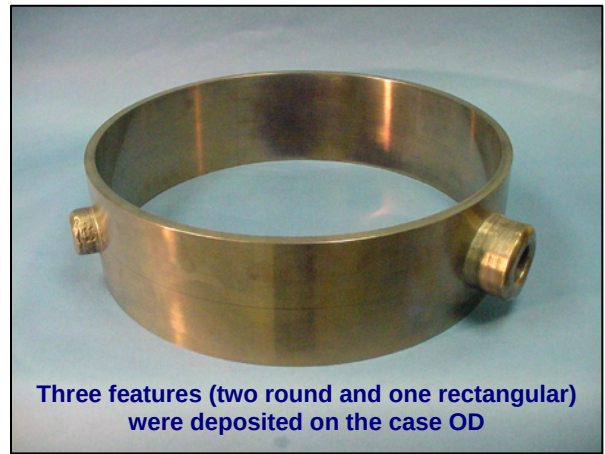
Figure 19: Images of P&W case that was fabricated from two 3" tall AMS 5662 rings EB welded together and machined to the nominal wall thickness of 0.5".
