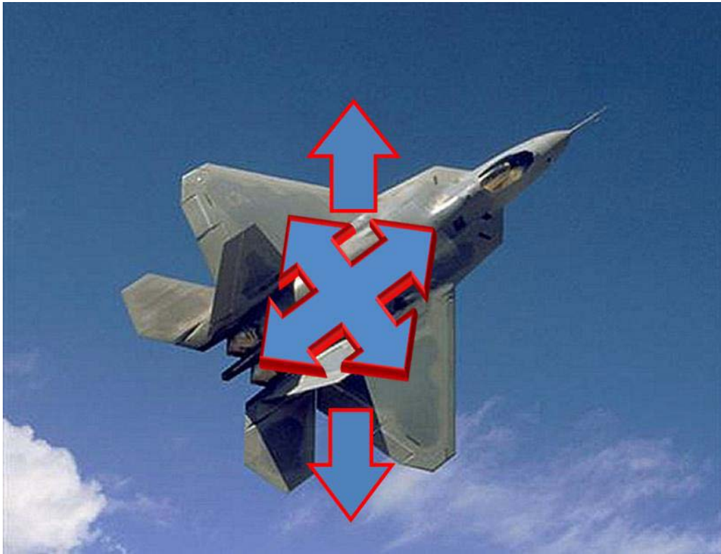
Figure 7.2.2-1 Vibration Axes during Combat Maneuvering
