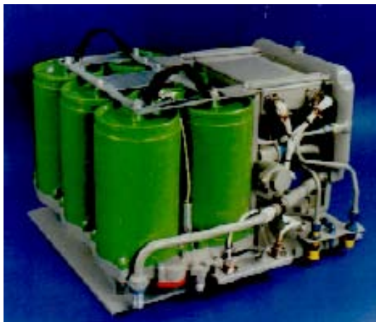
Figure 5.2.3-4. B-1B Oxygen Concentrator
