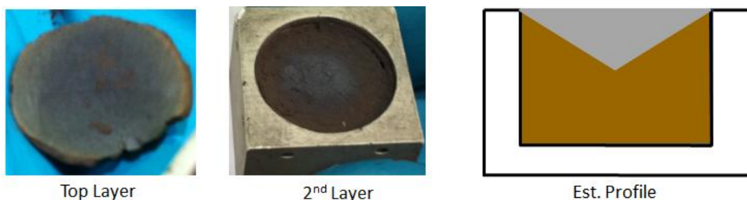
Figure 11. Discoloration pattern in the boron sample indicative of large thermal gradients.
