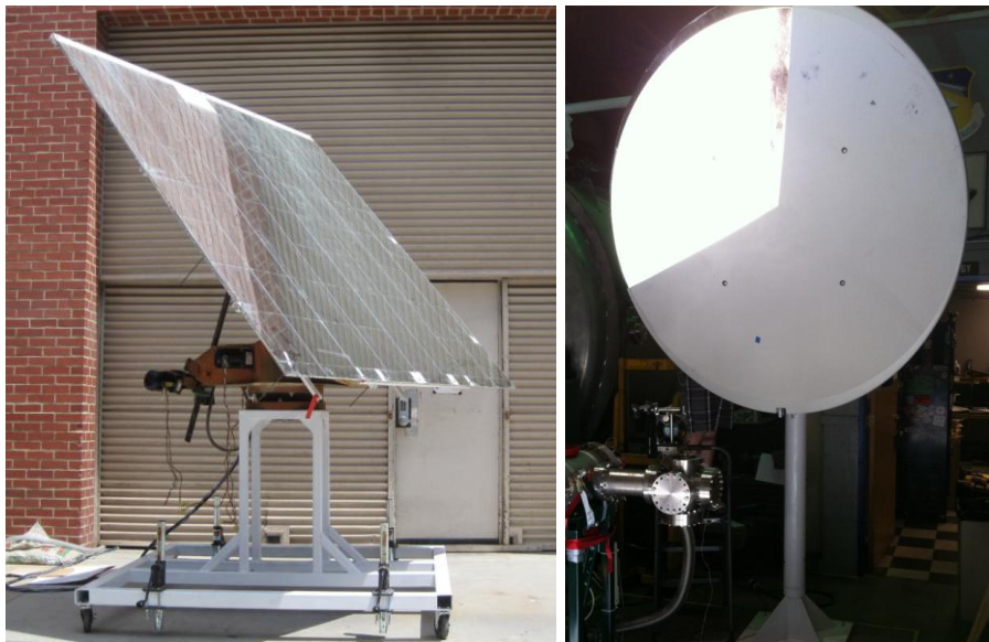
Figure 8. USC heliostat and partially mirrored 1.8 m offset parabolic concentrator.
