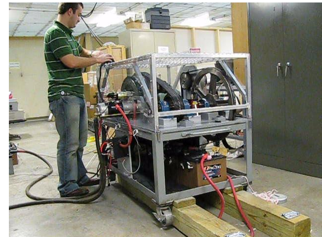
Hardware-in-the-Loop Test Bench (engine, starter, alternator)
