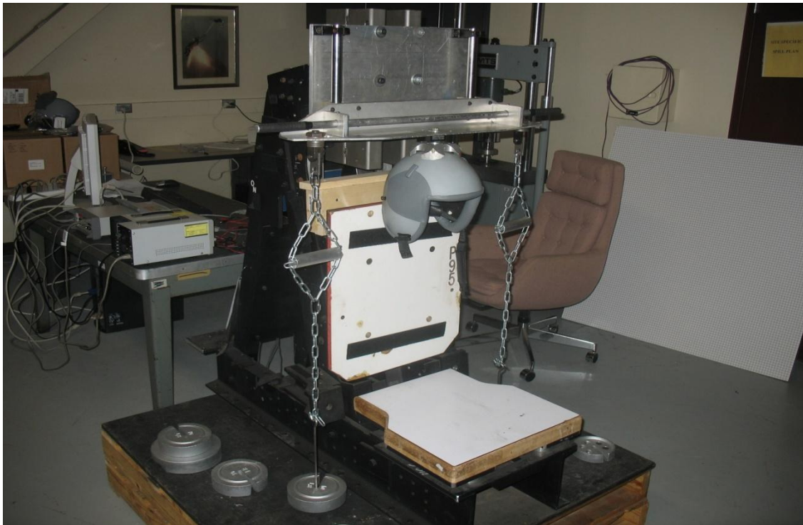
Figure 2. Neck strength test device test fixture
