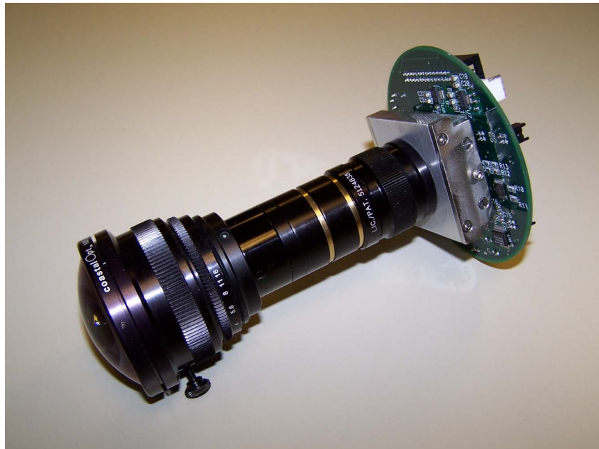
Figure 4: Side view of the camera assembly showing the fisheye lens, custom optical system, a translator for accurately positioning the image on the array, and camera electronics. The whole assembly is 16 cm long.
