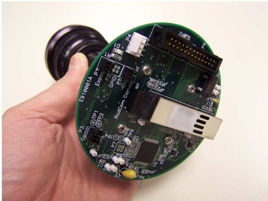
Figure 5: Picture of the backside view of the custom camera circuit board. The metallic box is the fiber transceiver.
