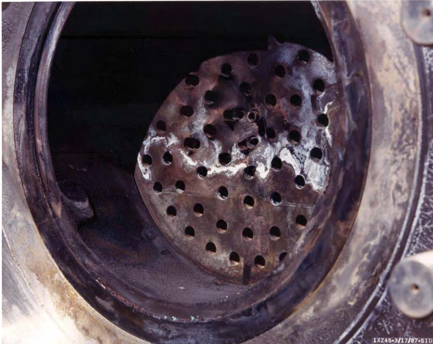
Damage to Rocket Chamber from Combustion Instability
