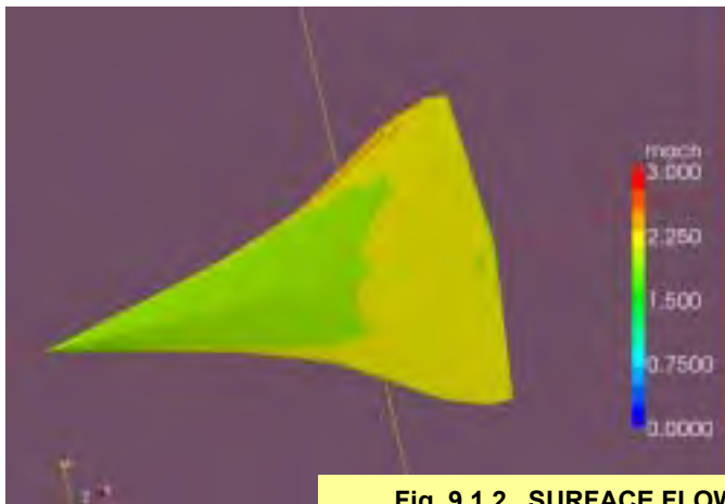
Fig. 9.1.2. SURFACE FLOW, Concorde Wing M 2.0, \alpha 4°, \beta 4°, Euler Method
