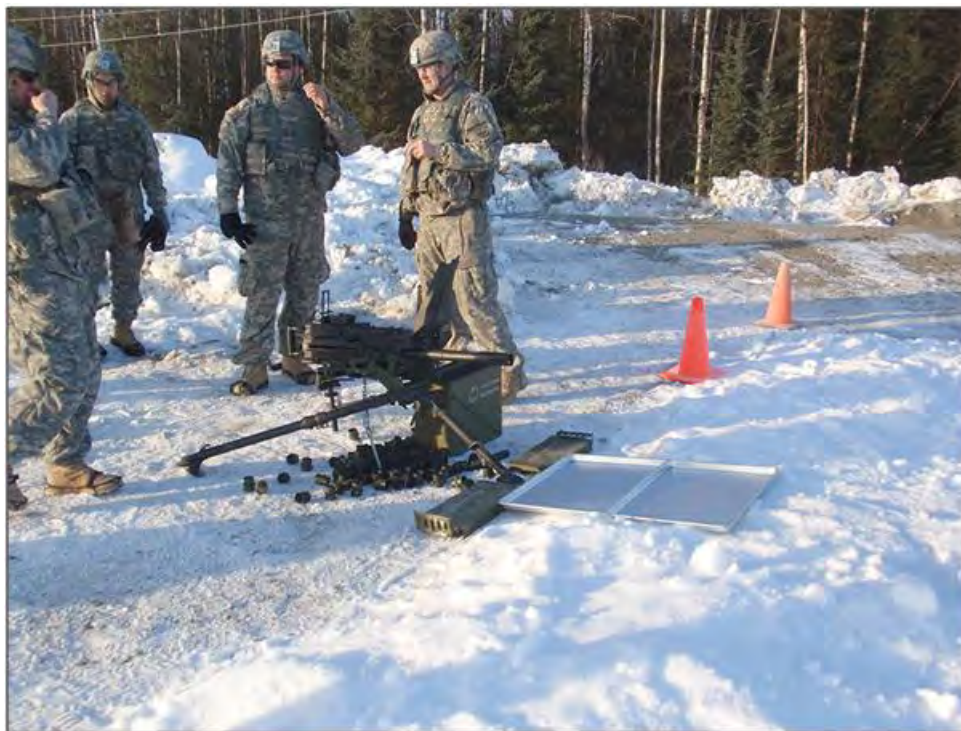
Figure 2-6. Location of trays used to collect propellant debris.
