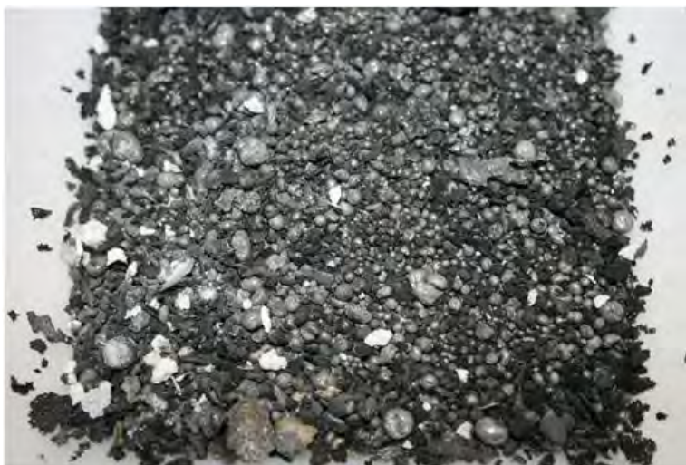
Figure 4-35. Close-up of the lead deposited in the burn table.
