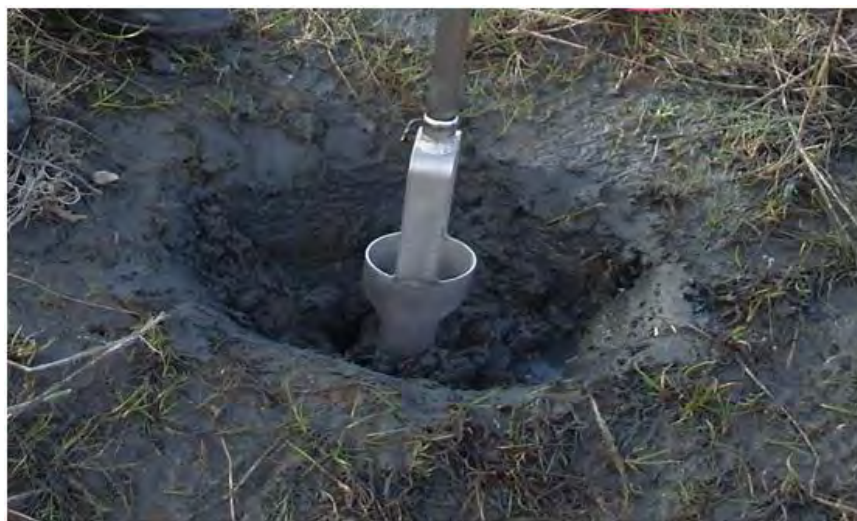
a. Top 15 cm of sediment was removed to prevent cross-contamination between the surface sediments and the subsurface.
