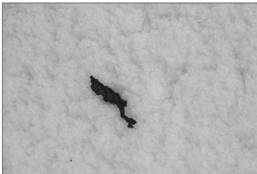
Figure 4-41. Representative large particle collected near the burning location.
