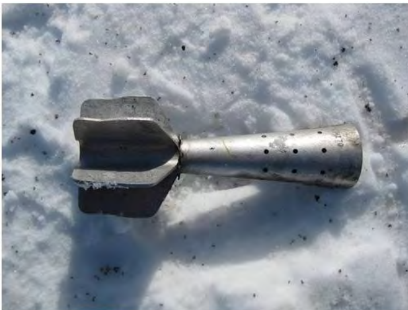
Figure 7-34. Tail recovered after sympathetic detonation of a UXO in test 9, round 9b (horizontal incoming round, 0.50-m distance).
