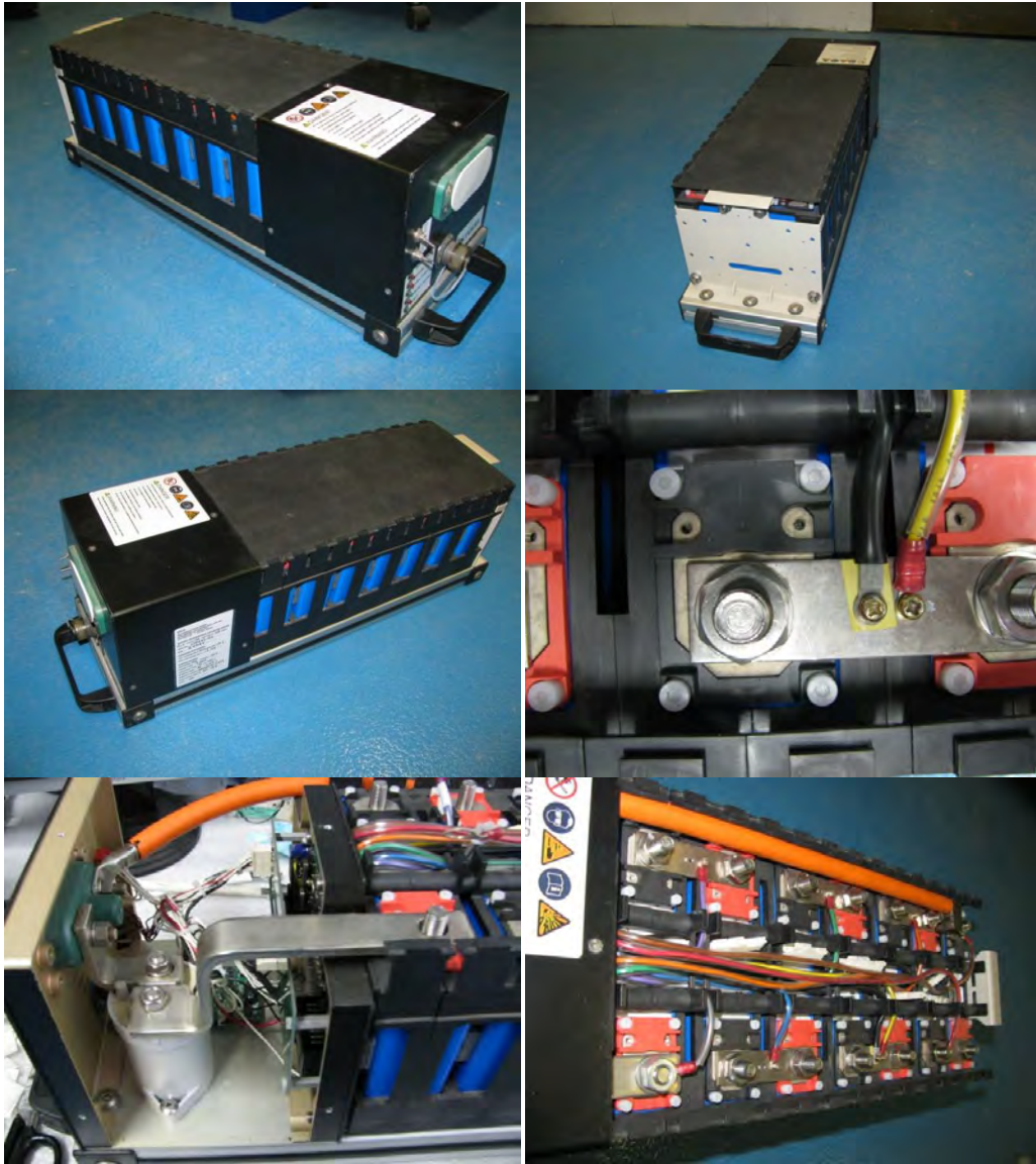
Figure 3 – Battery Module Disassembly Process Photographic Documentation: Left Side of Module (Upper Left); Back Side of Module (Upper Right); Right Side of Module (Middle Left); Close-up of Cell Buss bar and Temperature and Voltage Sensor Wires (Middle Right); Contactor and BMS Electronics Board (Bottom Left); and Module Complete Cell Stack (Bottom Right)
