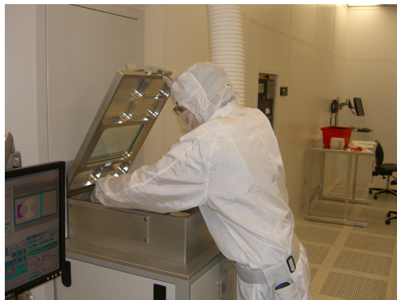
Figure 2.6: Carrier wafer being loaded into deep reactive-ion etching chamber.
