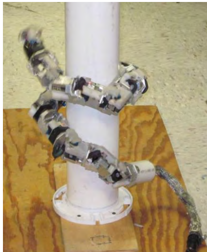
Figure 44. Examples of robotic snakes demonstrated during the program visit to CMU. The locomoting or free crawling snake (on the left) is observed climbing a pole. The surgical type snake on a moveable pedestal (on the right) can be directed to a location of interest.
