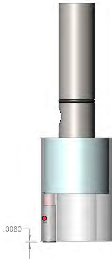
Figure A3: Design of the probe with a spring loaded coil. The .008 inch range is indicated.(Note that this entire probe is also gimbaled to allow for good seating during off-angle approaches.)
