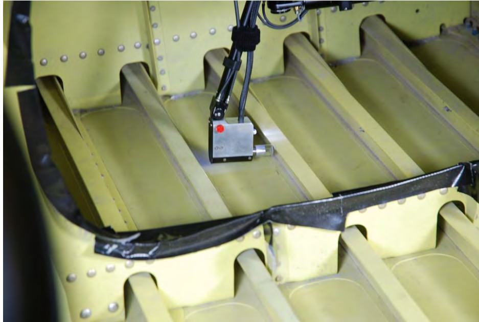
Figure 29. The SuNDE Tool micro eddy current scanner is shown moving into position for the selected A-10 inspection.
