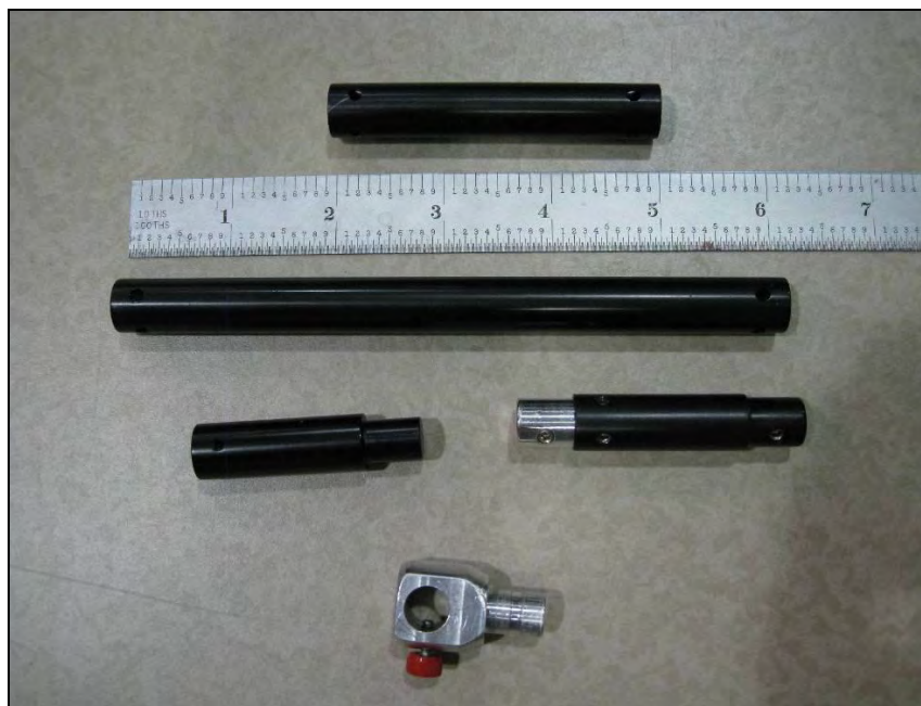
Figure 16. Various interchangeable lengths can be attached between the elbow and wrist as needed for the particular inspection scenario. A 90 degree fixture (shown at the bottom of the photo) can also be used if needed.
