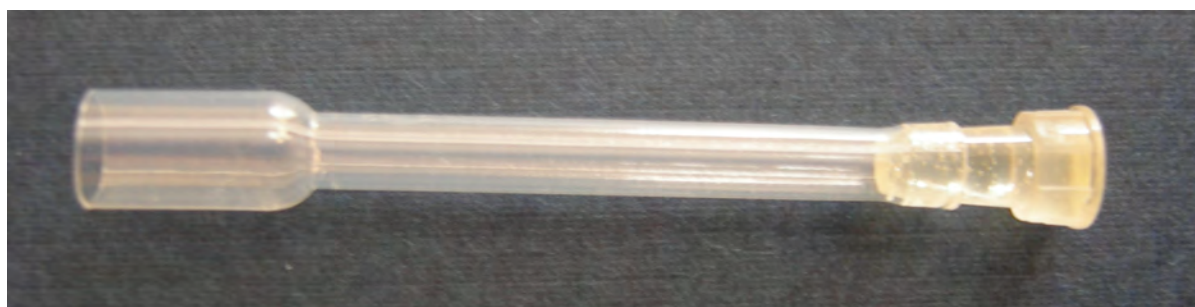
Figure 2 A photograph of a sample tube designed for storing tissue cultures. The sample tube was fabricated from a plastic transfer pipette.
