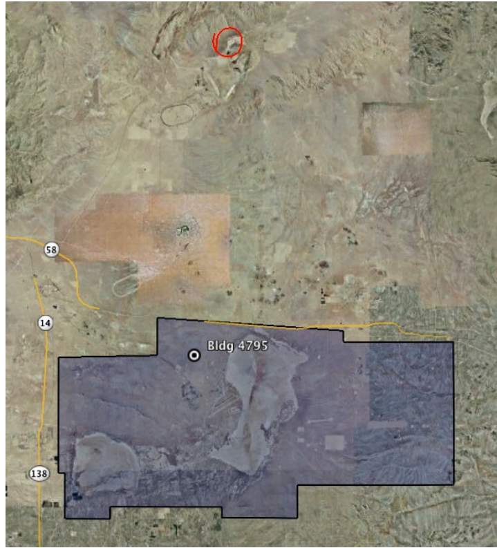
Figure 10: The flight path for test point M3 – a left-hand turn at a 30° bank. The flight path is the circle near the top of the image. The receiving site is the circle inside the shaded area.
