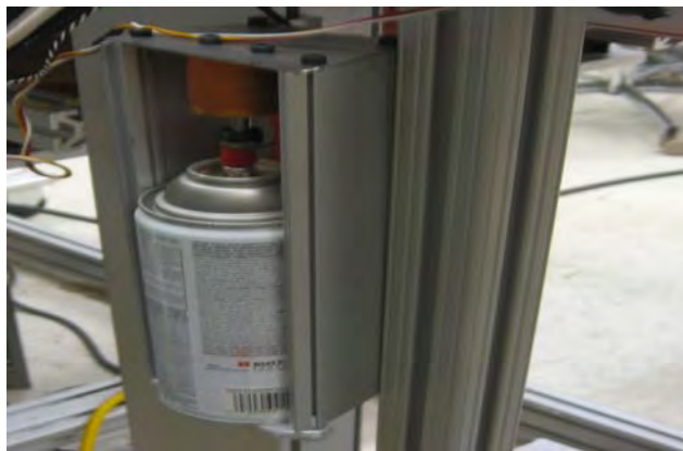
Figure A5.29. The pad labeling unit
