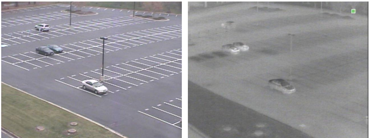
Figure 6. Example of a visible (left) and an LWIR (right) image in the FPSS dataset.
