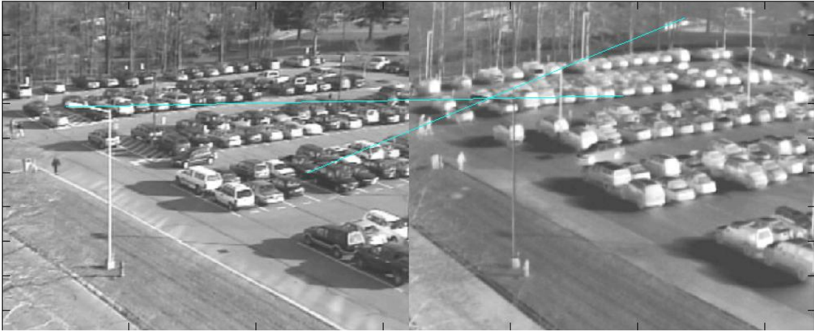
Figure 5. SIFT on visible and IR image frames showing few and inaccurate matches.
