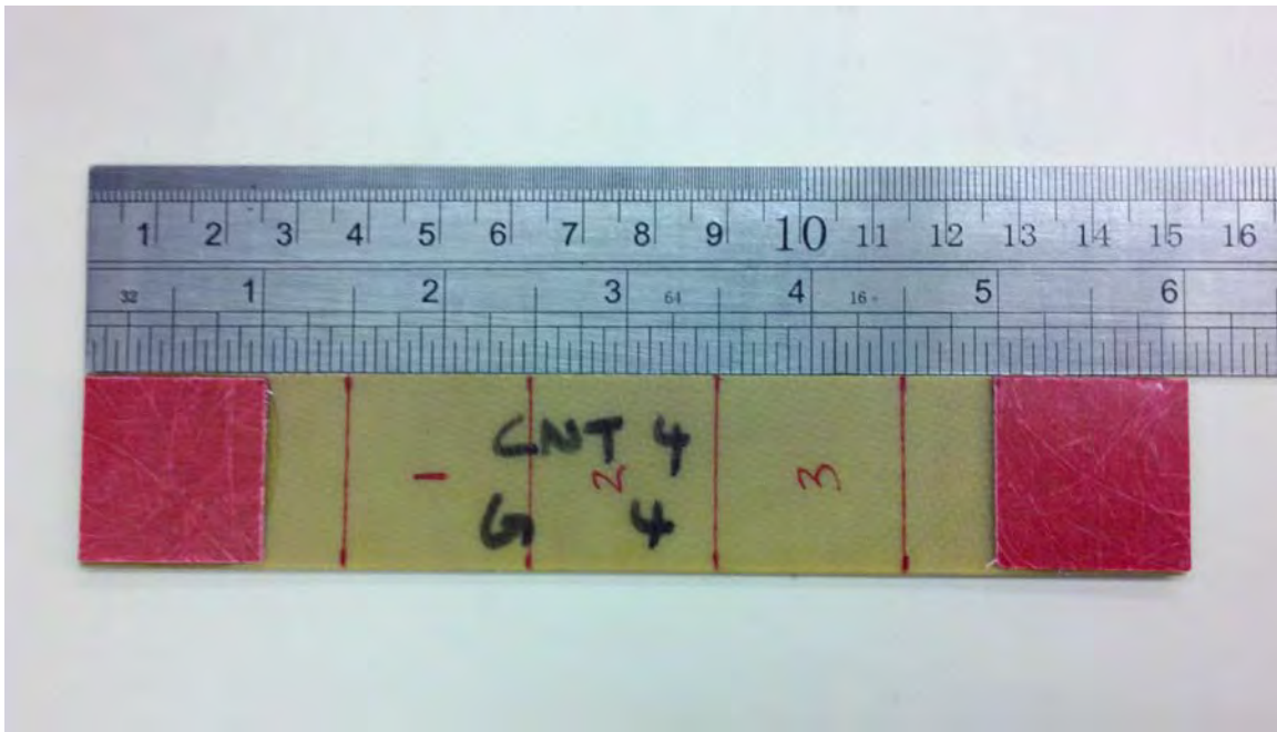
Figure 21. Test specimen divided into three sections for EMI measurements
