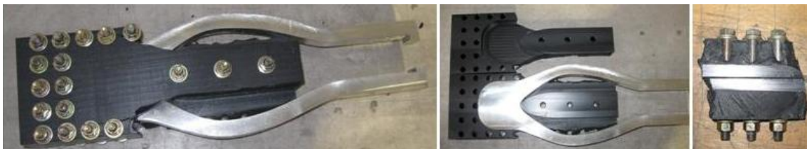
Figure 23. Post-test nylon bracket condition.
