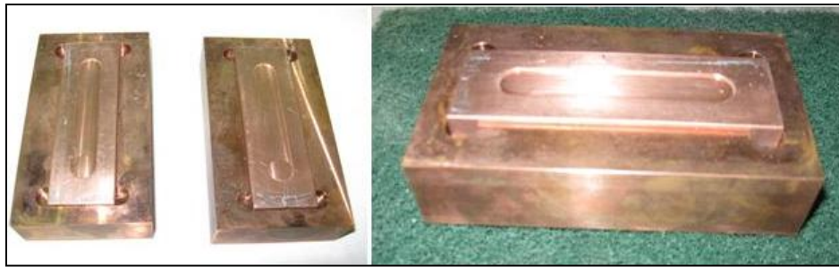
Figure 31. Full length pocket inserts in breech blocks.
