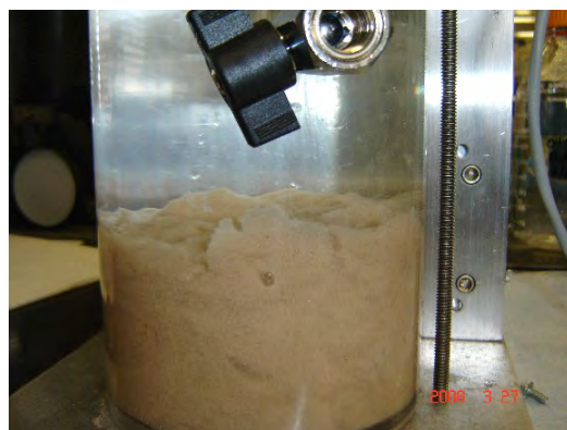
Figure 75. Plain Sand Resuspension at 3.7 m/s (A) and Erosion at (11 m/s) (B).
