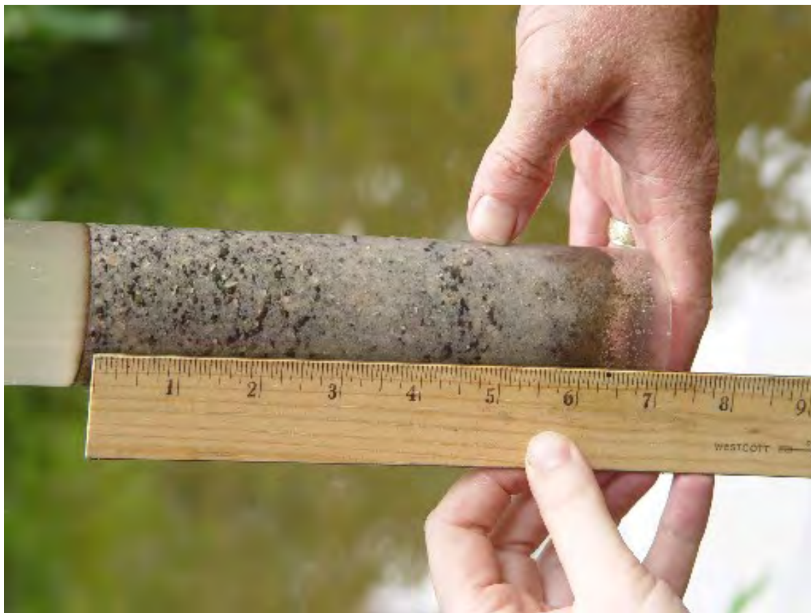
Picture 20. The Average Cap Thickness was about 6 Inches.
