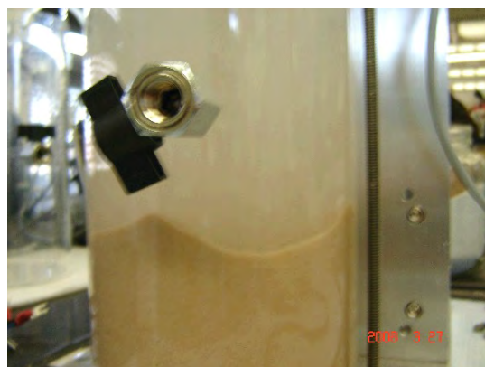
Figure 75. Plain Sand Resuspension at 3.7 m/s (A) and Erosion at (11 m/s) (B).
