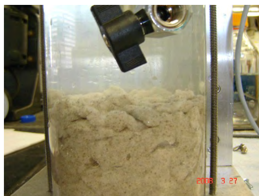
Figure 76. Coated Sand with Xanthan and Guar Gum did not Erode at 3.7 m/s (A) or 11m/s (B).
