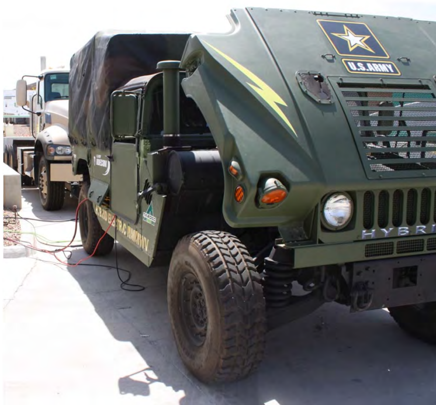
Diesel-Electric Hybrid High Mobility Multipurpose Wheeled Vehicle (HMMWV) in Exportable Power Demonstration at Ft Bliss, TX during the 2010 Renewable Energy Rodeo & Symposium
