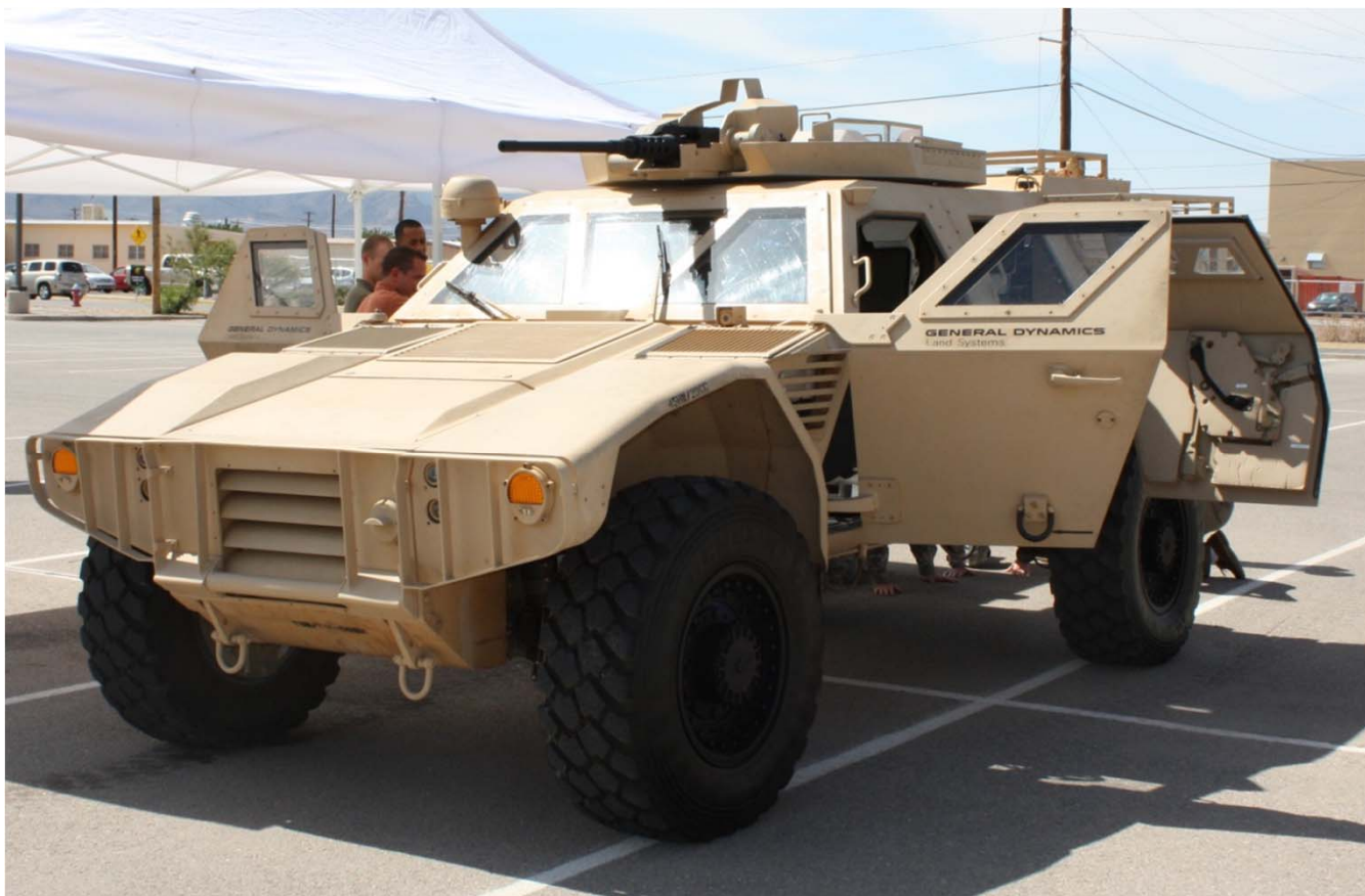
Diesel-Electric Series Hybrid Advanced Ground Mobility Multipurpose Vehicle (AGMV) in Display/Ride/Drive at Ft Bliss, TX during the 2010 Renewable Energy Rodeo & Symposium
