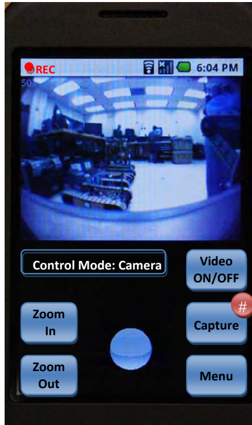
Figure 8. When the camera mode is chosen, camera controls are displayed. These camera controls include both video and still photographs. Video recording status (i.e., currently recording) is shown in the upper left corner on the status bar. The number of still images taken (or some other information) can be identified in a small area on the screen as well.
