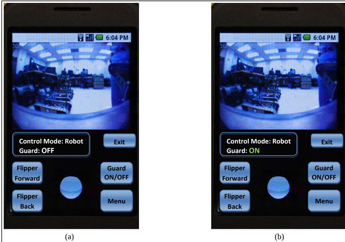
Figure 10. Concept for adding the ability to turn the guarded teleoperation function on and off. (a) Tele-operation guard is OFF (i.e., pure teleoperation without obstacle avoidance). (b) Tele-operation guard is ON (i.e., obstacle avoidance is being used).
