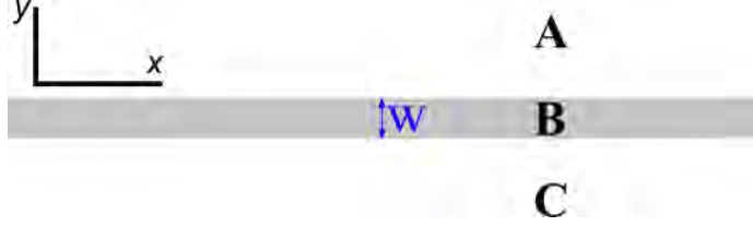
Figure 5-4: Idealized wave constructed by the two sharp vertical interfaces separated by distance W .
