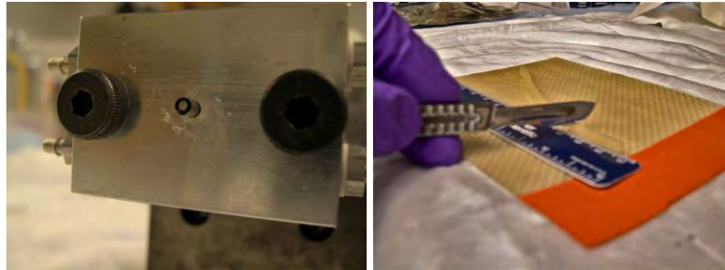
Figure 5: (left) An albumin tube being extruded. (right) Stents being cut into 17 mm sections with a scalpel.
