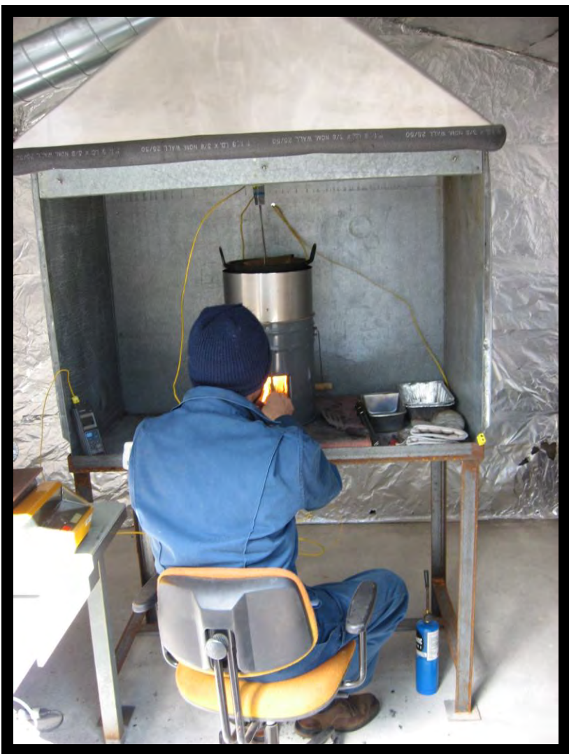
Stove testing in emissions hood
