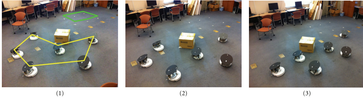
FIGURE 12: Three sequential snapshots of the 6 iRobot Create robots executing the motion planner presented in this paper. The first frame shows the connectivity ring and the goal positions.
