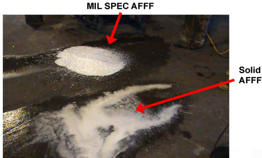
Figure 7. Aerated MIL-SPEC AFFF compared to solid AFFF.
