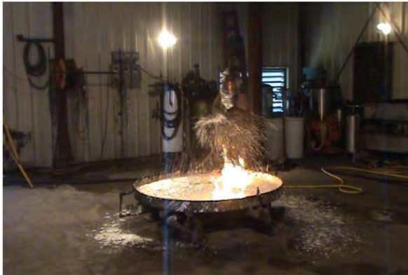
Figure 9. Comparison of fire knockdown between MIL-SPEC AFFF and 3M solid pellet AFFF.
