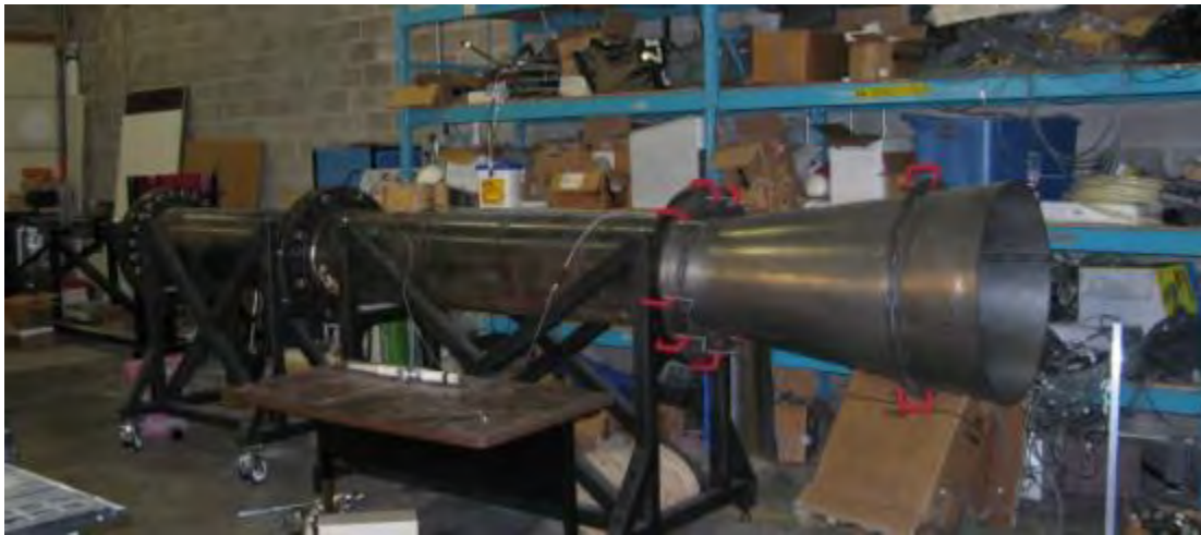
Figure 2.1.3.5-1. 18-inch diameter shock tube.
