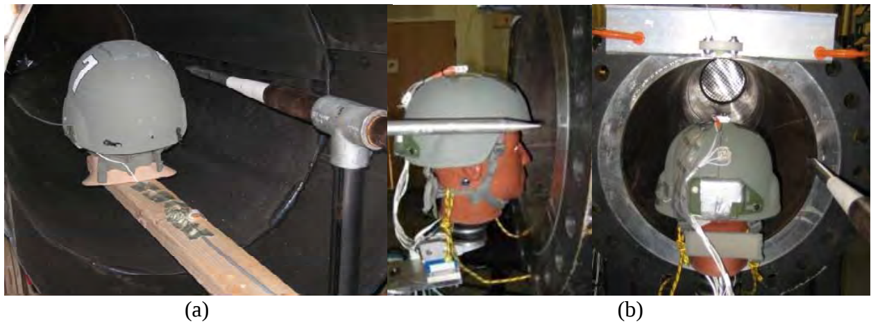
(a) (b) Figure 2.3.1.1.3-3. FOCUS head and neck with helmet positioned (a) in cone for long duration blasts and (b) at the end of the ARA shock tube.
