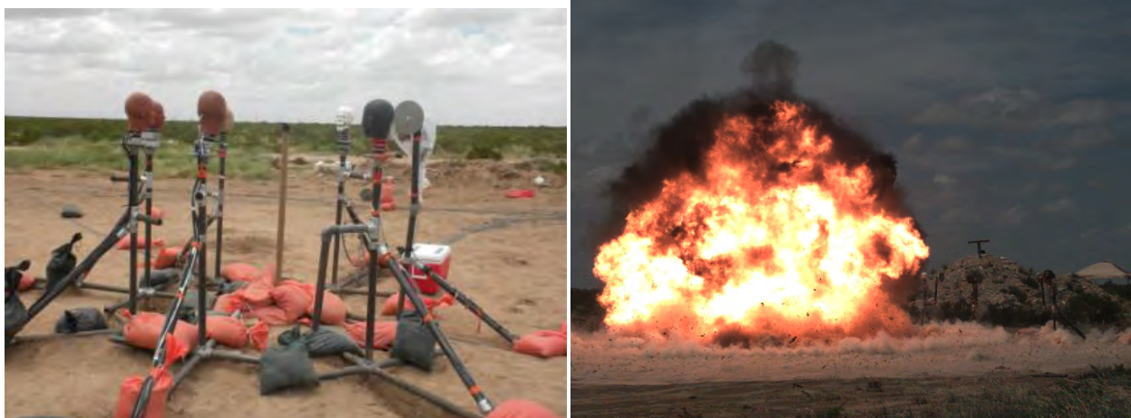
Figure 2.4.1-1. (left) Test arena with 7 headforms. The standoff distance was 42 inches. (right) blast event from the test series,
