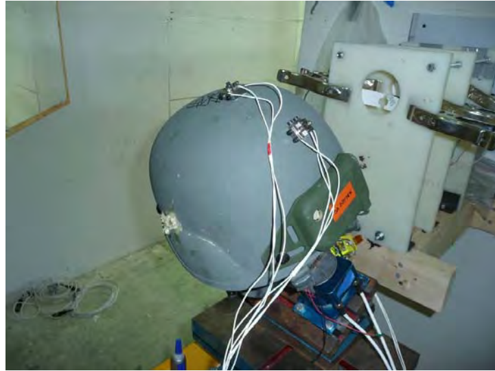
Figure 2.3.2.3.1-2. View of test helmet in side orientation, showing rear of helmet and Med-Eng sensor.
