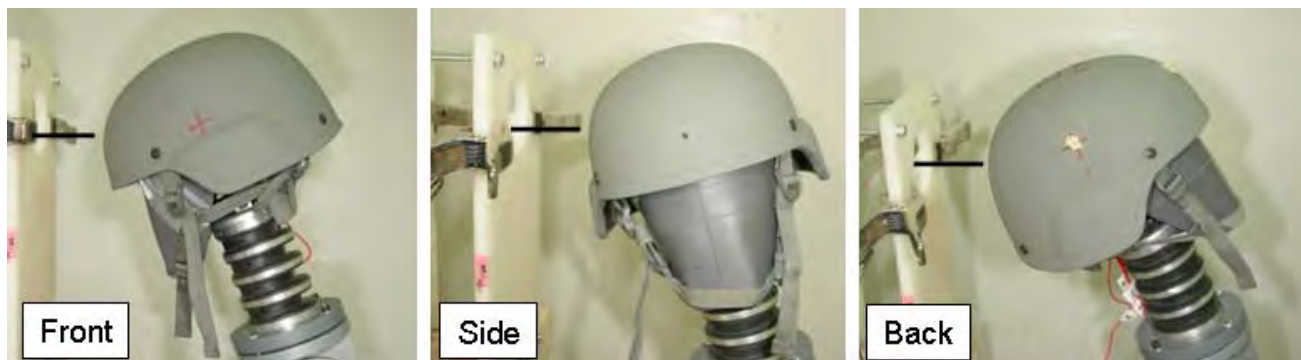
Figure 2.3.2.1-9. Representative Impact Locations on the ACH Helmet
