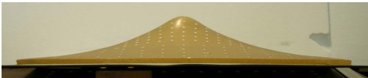
Figure 10 Example of a coated plate after the experiment (4 mm D36 plate with 10 mm coating)
