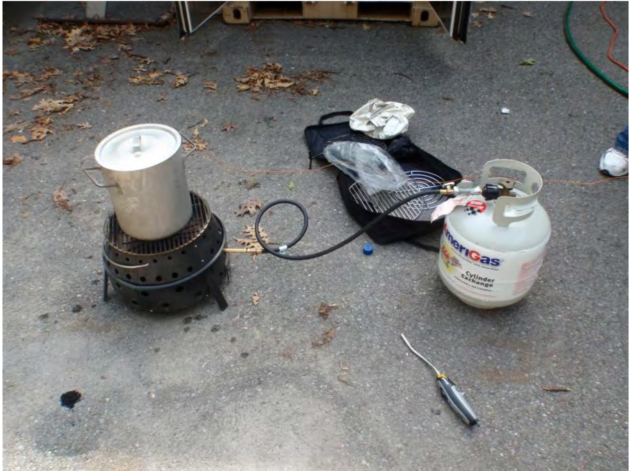
Figure 11. Propane Boil Test-2.5 Gal-Top Grate-No Baking Lid
