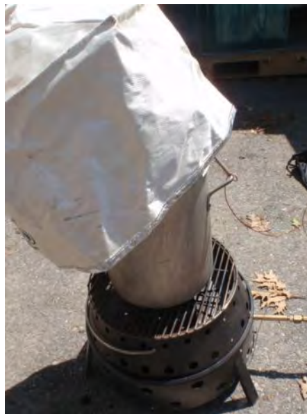
Figure 13. Propane Boil Test-Top Grate-With Baking Lid
