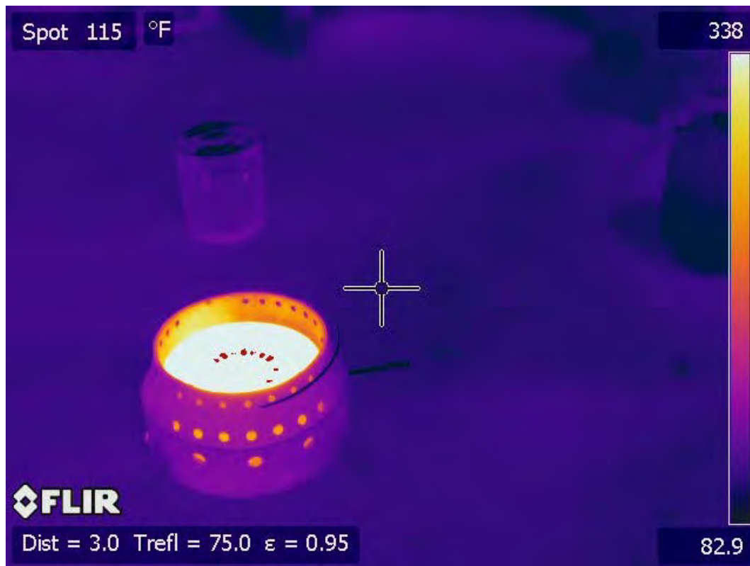
Figure 25. Thermal Image of Volcano II Stove Operating With Propane under Wind Test Conditions
