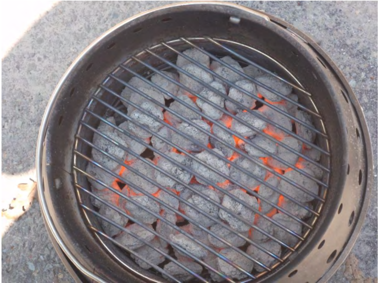
Figure 26. Volcano II Stove Operating With Charcoal under Wind Test Conditions
