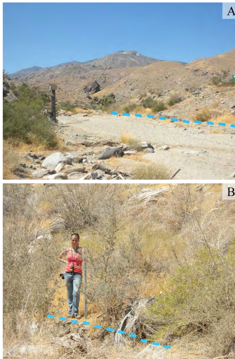
Figure 33. Palm Canyon Wash, with the field OHWM shown by the blue dashed line: (A) view upstream towards the gage, and (B) eroded slope below the field OHWM.
