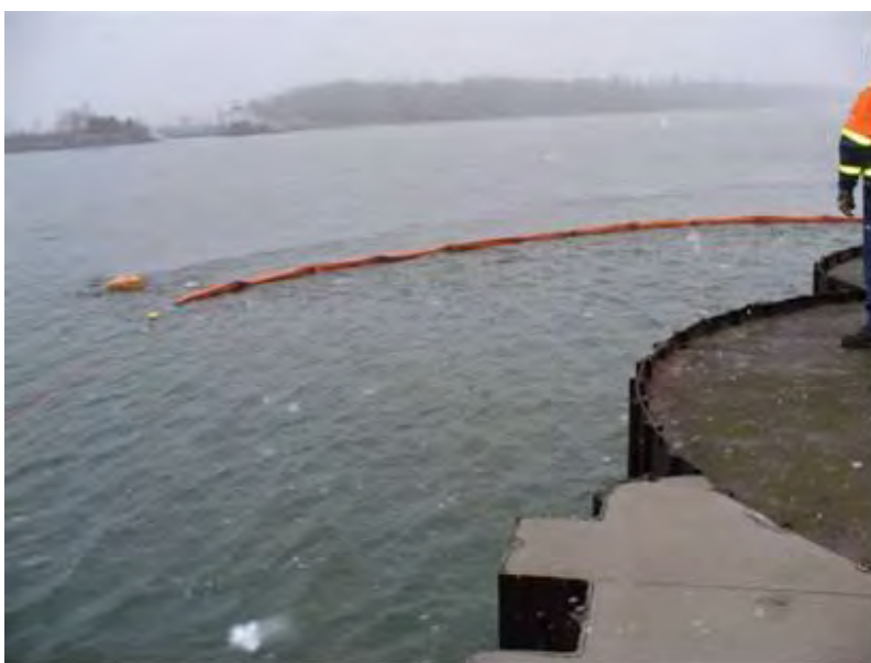
Figure 17. Boom Vane controlling boom.
