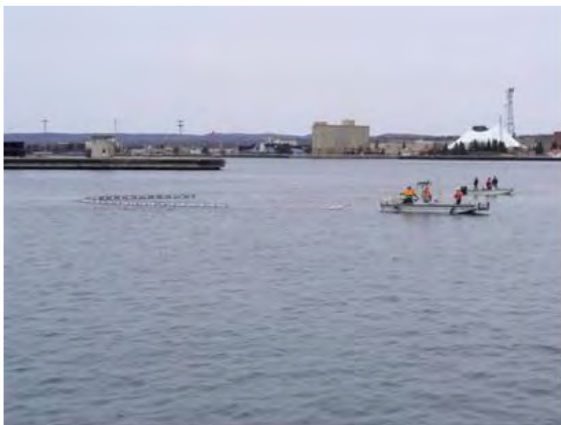
Figure 7. PyroBoom being towed in containment configuration.
