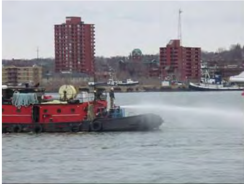
Figure 9. Fire monitor in use.
