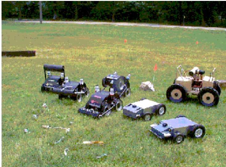
Figure 1. Basic UXO Gathering System (BUGS) Prototype Robots
