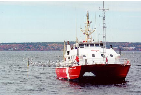
Figure 3: SWATH ship Frederick Creed fully configured for the Shoaling Waves Experiment during sea trials in Bedford Basin, Nova Scotia. Figure 4: A close-up view of the SWATH ship
