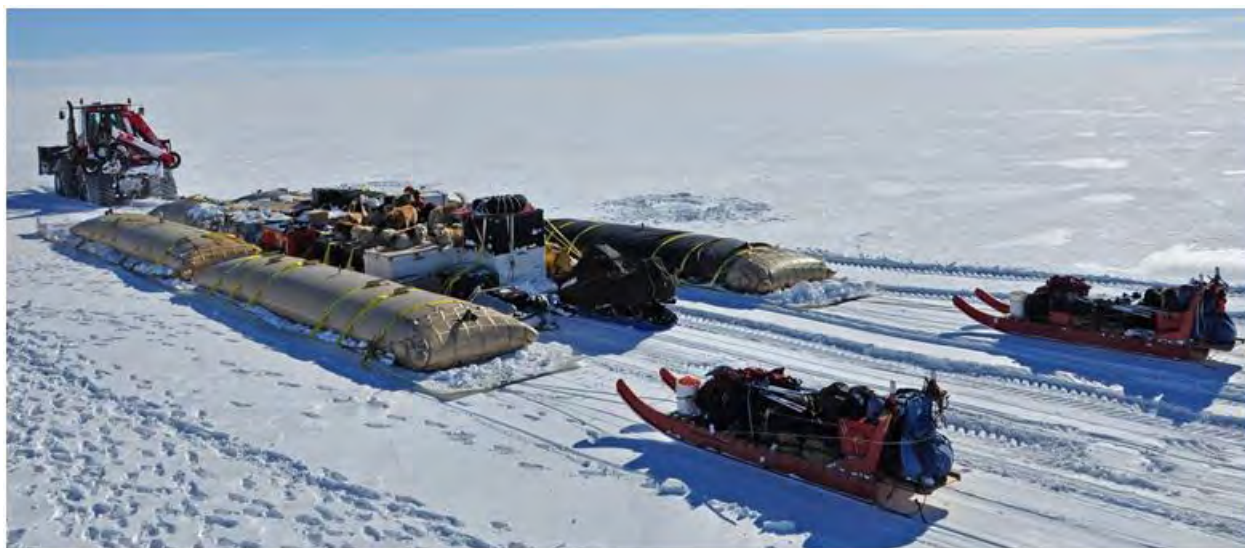
Figure 5. Case Quadrac towing full load of dual-3000-gal. bladder sleds on either side of a Dura-Base cargo sled. The left-side bladder sled included electric blankets under both bladders, while both bladders on the right-side sled were wrapped in black covers. The photo (courtesy Robin Davies) shows Go North dogs and sleds catching a lift en route to NEEM.
