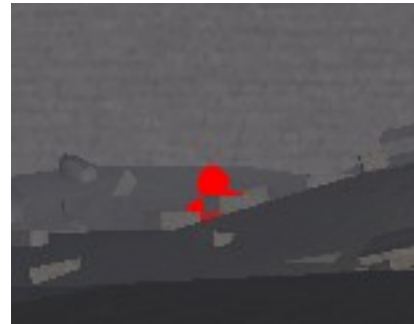
Figure 10: Although the color of the target is a striking contrast to the background, its intensity is similar, leading ACQUIRE to predict a nearly zero (.0004) detection probability. Note that this is a detail of the actual image presented to the subjects and not a false color image!
