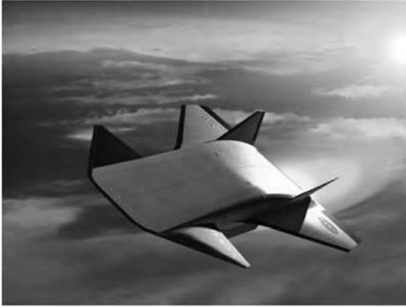
Fig. 1 NASA X-43B showing canard and elevon control surfaces.
