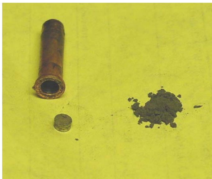
Figure 2. Photograph of igniter mixture candidate 12 as both powder and pellet. Flash tube is also shown.
